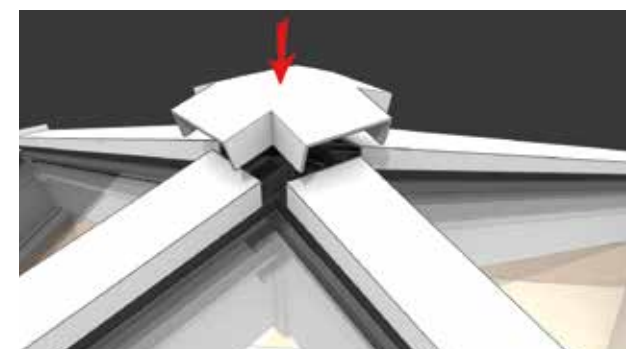
23 Push down central cross cap so it locates firmly onto the top of the pressure plate.
