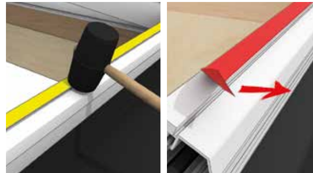
14 Clip trim onto the top of the ringbeam using a rubber hammer if required and then peel back the corner of the protective tape and fully remove.
