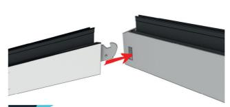
Loosen retention screws in hips and insert the connection brackets into the wider machined slots in the side of the ridge. Return to step 8, fitting the framework into the ringbeam, pushing down the hips to tighten the joints. Tighten retention screws.
