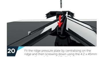
screws through the pre-drilled holes.
