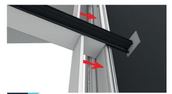
Use internal foamboards to space out rafter positions before fixing rafters to the ringbeam.
