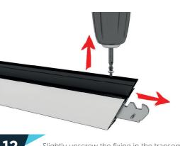
2 Slightly unscrew the fixing in the transom rafter or jack rafter to release the connection bracket.
