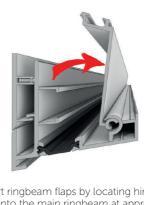
Insert ringbeam flaps by locating hinge part of the flap into the main ringbeam at approx 80 degrees as shown, then rotate forward to lock in.
