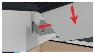
Lift transom rafter and offer the bracket up to the slot in the ridge at an angle. Insert the bracket and then rotate the rafter into position at the ringbeam.
