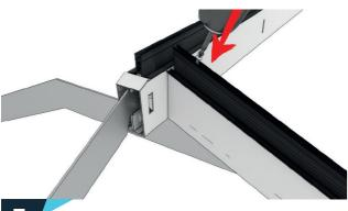
Re-tighten bracket retention screw to pull the ioint tight.
