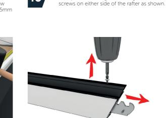
Slightly unscrew the fixing in the transom rafter to release the connection bracket.
