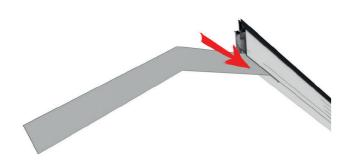
Insert tie bar bracket into the side of one of the central rafters.
