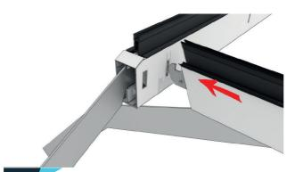
2 Loosen retaining screw from transom connection bracket so that it can move freely and insert transom bracket into slot in the ridge.
