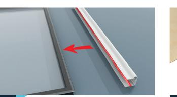
Apply a bead of sealant to glazing end closer and fit centrally to glass units.
