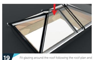
Fit glazing around the roof following the roof plan and sit against the lower endcaps. If a roof vent has been specified, follow roof vent installation. Apply pressure to the adhesive of the glazing tape to secure the glass.
