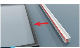
Apply a bead of sealant to glazing end closer and fit centrally to glass units.
