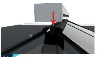
Fit the ridge top cap in place by centralising and applying pressure from one end to the other.
