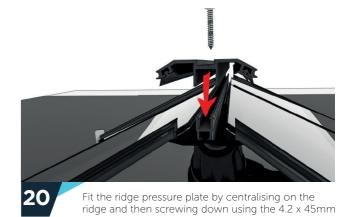
ridge and then screwing down using the 4.2 x screws through the pre-drilled holes.
