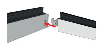
Loosen pre-fixed top bracket screw and slide hip rafter and top bracket into slot provided in the ridge body.
