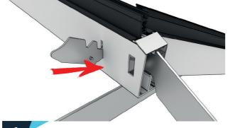
Insert the transom connection bracket into the slot in the opposite side of the ridge.
