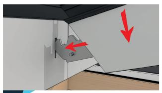
Lift transom rafter or jack rafter and offer the bracket up to the slot in the ridge or hip at an angle. Insert the bracket and then rotate the rafter into position at the ringbeam.
